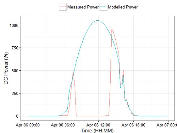
**Figure 9:** Measured and modelled power of a PV system during the FDR testing phase.
