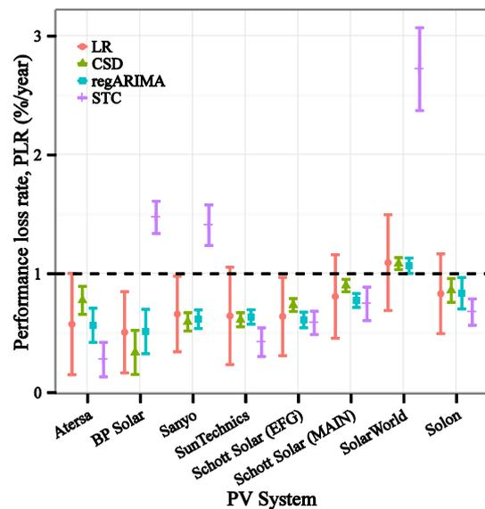
Figure 8: Annual performance loss rates evaluated through outdoor time series analysis for the evaluation period June 2006 – October 2014 and indoor testing at STC. The 1 %/year line is used as a visual aid [10].
