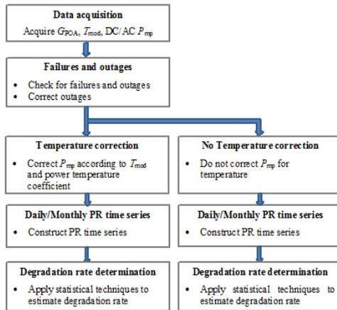
**Figure 3:** Degradation rate determination algorithm procedural flow chart.
