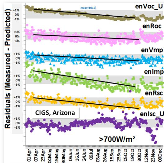
Figure 7: Degrading performance of a CIGS module in Arizona analysed with the LFM.
