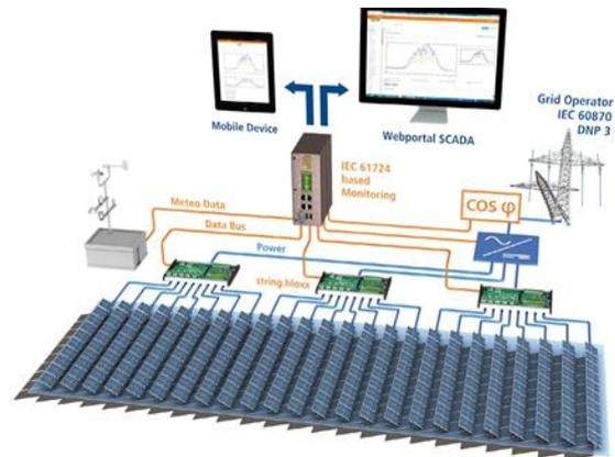
Figure 2: Outline of the advanced monitoring system installation for large scale PV plants.
